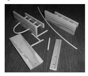
Fig 5, shows an assembled seat and the components that are required to make the seat. Once the seat is assembled it can be installed into the Coracle frame.
